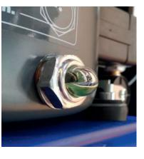
Refill the oil **(A)** using the funnel supplied in the tool kit **(E)**.
