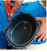
Remove the O-ring joint **(D)** which enables the sealing of the cylinder head.
