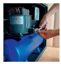
Once the compressor is empty, unscrew the oil indicator with a 27 mm socket wrench **(3)**.
