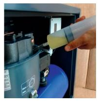
Insert one end of the pipe into the syringe cap **(E)**. Then, thread the other end to the bottom of the compressor block. Suck up the oil using the syringe
