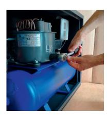
Place the copper washer **(C)** on the oil indicator **(C)** and screw it back on with the 27 mm socket wrench.
