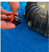
Unscrew the vacuum breaker **(B)** / **(2)** and replace it.
