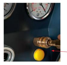
Drain the vacuum using the vacuum plug, by connecting the male connector without the hose.
