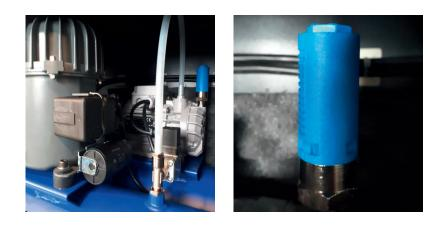
Unscrew the discharge silencer (H). Only the blue plastic body must be unscrewed. Insert the new discharge silencer from the annual maintenance kit (H).
