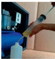
In removing the hose, dry the end with a rag. Empty the liquid into the empty bottle provided for this purpose **(E)**. Repeat until all the oil has been removed
