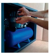
The four screws must be tightened diagonally and progressively.
