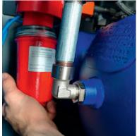
Replace the filter element with the new cartridge received in the kit (G). Peel off the «Service Rule» label on the bottom of the filter.
