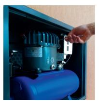
Unscrew the 4 screws **(14)** securing the cylinder head **(16)** of the compressor block.
