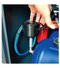
Open the access panel using the supplied key. pull up the two black tabs that secure the vacuum filter cover **(F)**
