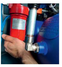
Unscrew the lower part of the filter body (red). Remove the filter cartridge by pulling down with a slight rotary motion.
