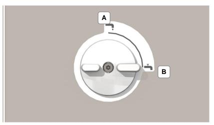
Illustration 4.7 View turning knob for draining the tank
